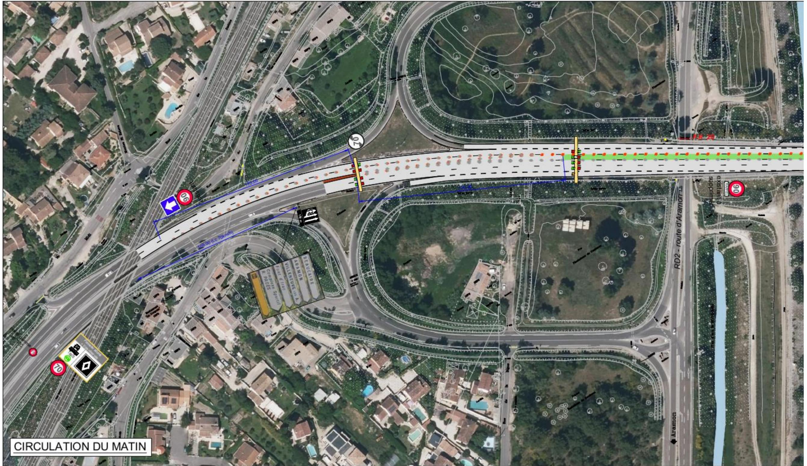
FIGURE 15 PLAN MASSE DEBUT DE VOIE REVERSIBLE A L'HEURE DE POINTE DU MATIN, ETUDE PRELIMINAIRE, EGIS
