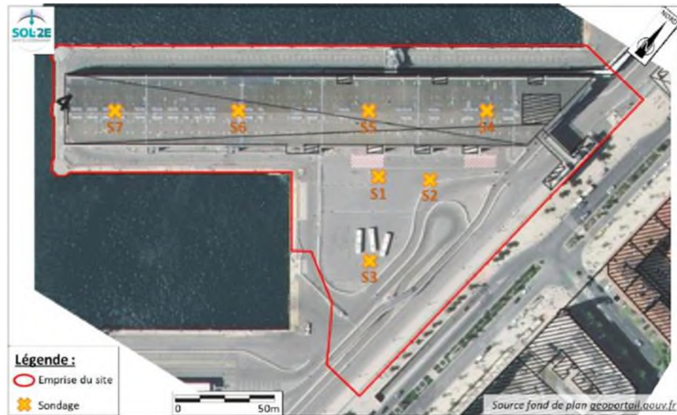
Figure 64 - Sondages de sols (SOL-2E)
