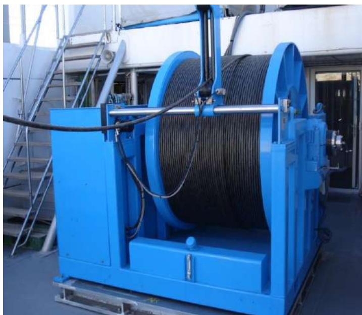
Figure 5. Treuil de manutention hydraulique.
